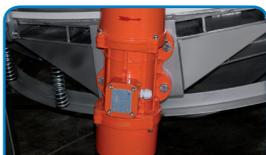
Driven by laterally attached vibration motors (ATEX 22)
